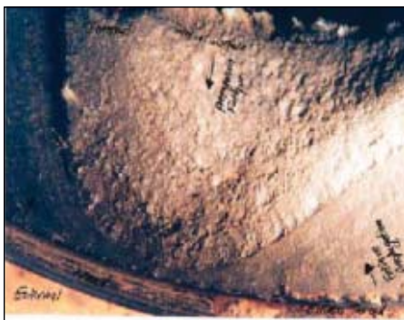
Macroscopic view shows two fatigue cracks initiated from external and internal jar surfaces. Highly deformed fatigue cracks are visible (Fig. 5).
