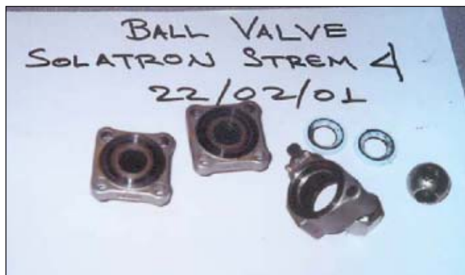
The photograph on the left shows parts of a ball valve from the feed line of an online densitometer heavily contaminated by black powder. The right photograph shows the inlet filter element of a similarly contaminated online densitometer (Fig. 6).
