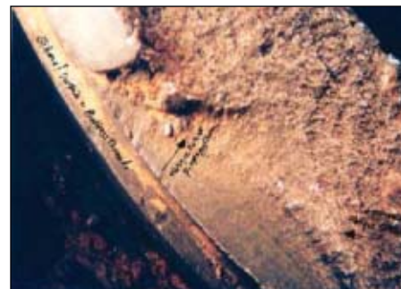
Macroscopic view shows two merged fatigue cracks resulting from high drilling torque (shear stress) during drilling operations (Fig. 4).
