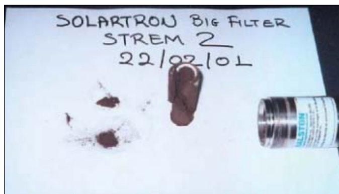
The photograph on the left shows parts of a ball valve from the feed line of an online densitometer heavily contaminated by black powder. The right photograph shows the inlet filter element of a similarly contaminated online densitometer (Fig. 6).
