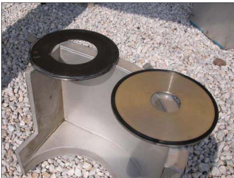
Black powder thoroughly coated the orifice plate shown on the left of this photograph. A clean orifice plate provides contrast (Fig. 2).
